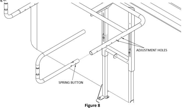
9. Swing the U-Arms up so that they are parallel to the ground. Raise the Main Unit so that the bottom tube of the U-Arms is level with the top of the spa without the cover. See Fig 9.
